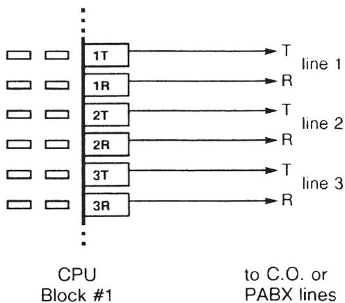
1. Connect Tip and Ring of each line to the associated *T* and *R* pair on the right side of CPU block #1.
