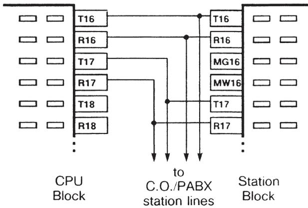
Connect *T* (Tip) and *R* (Ring) from each monitored station to the associated *T* and *R* pins on CPU block #2 or #3. The 1030/1560 is connected in parallel with the station lines.
