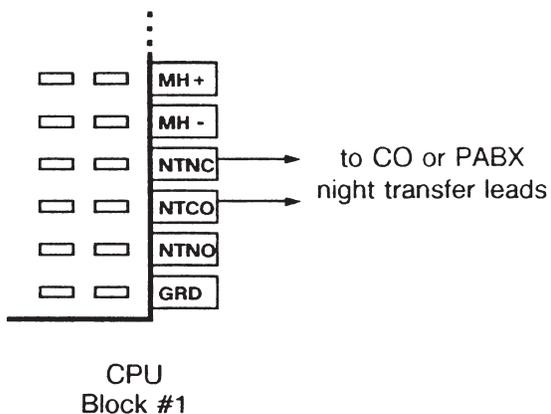
Connect *NTCO* (common) and *NTNC* (normally closed) on the right side of CPU block #1 to the night control terminals on the telco/PABX block.
