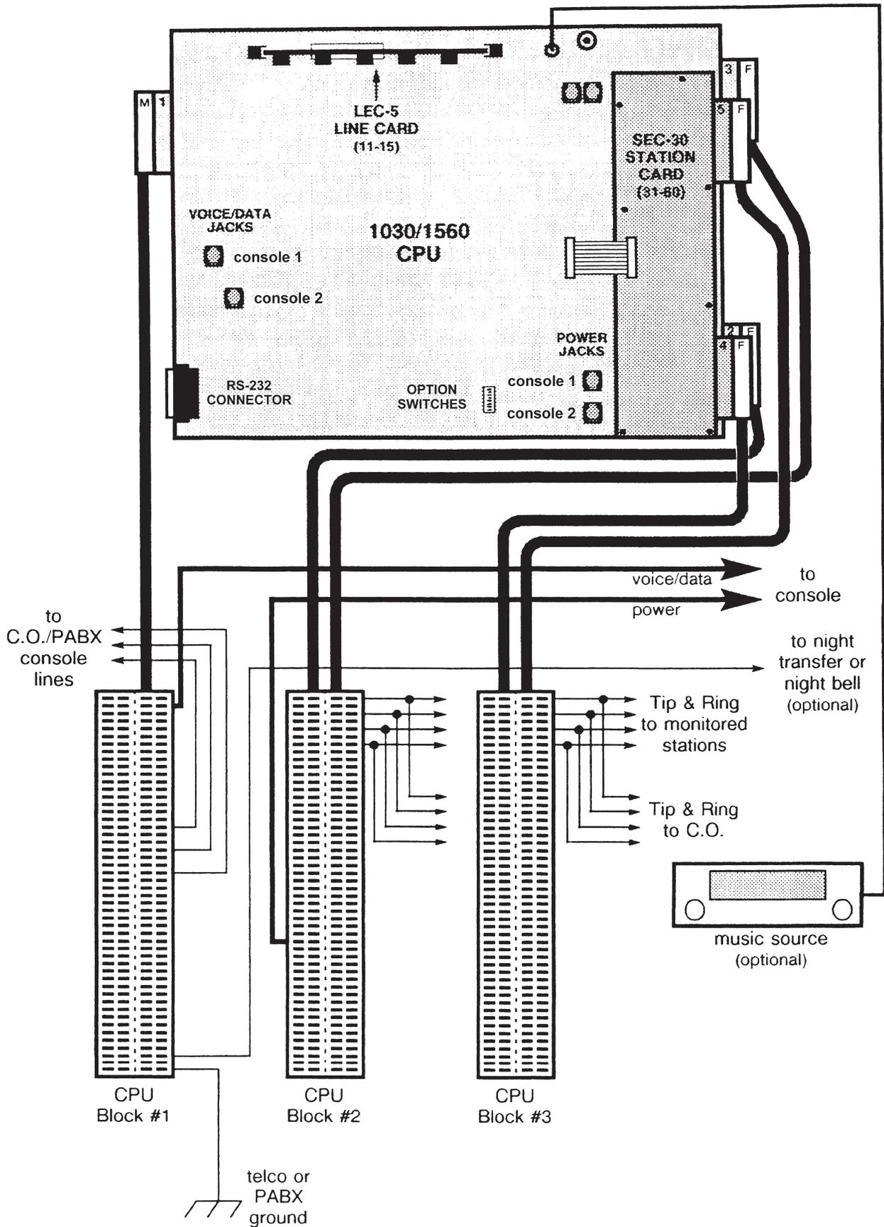
Figure 5 – 1030/1560 Typical Installation
