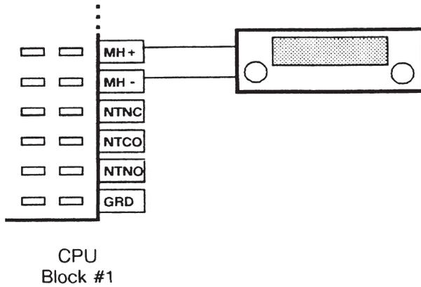
1. Connect a twisted wire pair to *MH+* and *MH-* on the right side of CPU block #1.
