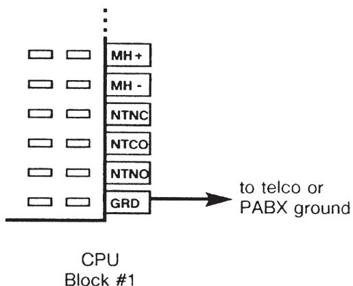
Connect telco or PABX ground to the GRD pin on the bottom right of CPU block #1.
